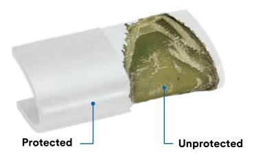
Sample tested in rainfall of one inch per hour at 500 mpg at the University of Dayton Research Institute Rain Erosion Test Facility.
